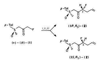
Scheme 1. i, Lithium di-isopropylamide (2.2 mmol)/THF/-78 °C; ii, allyl bromide (1.5 mmol)/THF/-78 °C; iii, chromatographic separation (pentane-diethyl ether, 4:6)
