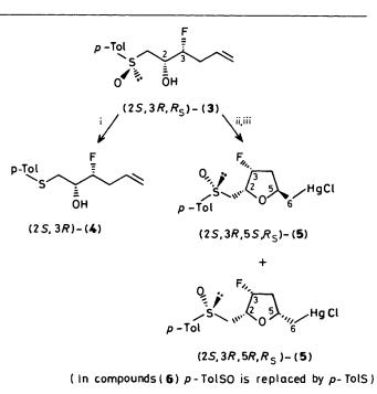
**Scheme 2.** i, Sodium iodide/trifluoroacetic anhydride/acetone/-40 °C; ii, mercury(II) trifluoroacetate/THF/0 °C; iii, potassium chloride/water
